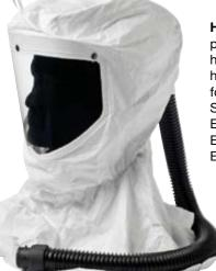
**Hood SR 561** A lightweight hood which protects head and shoulders. Replaceable hood of Tyvec with an easily adjustable head harness. Easily adjustable and comfortable neck seal of cotton. Visor of PETG. SR 561 is TH3 approved in accordance with EN 12941:1998.
