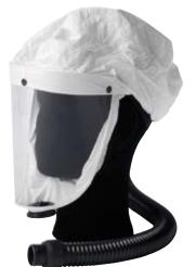
The face shield and the hoods are delivered with hose for direct assembly in SR 500 EX. **Hood SR 562** A lightweight hood which covers the face and head. Replaceable hood of Tyvec with an easily adjustable head harness. Available in one size. Easily adjustable and comfortable face seal in polyamide/lycra. Visor of PETG. SR 562 is TH3 approved in accordance with EN 12941:1998.
